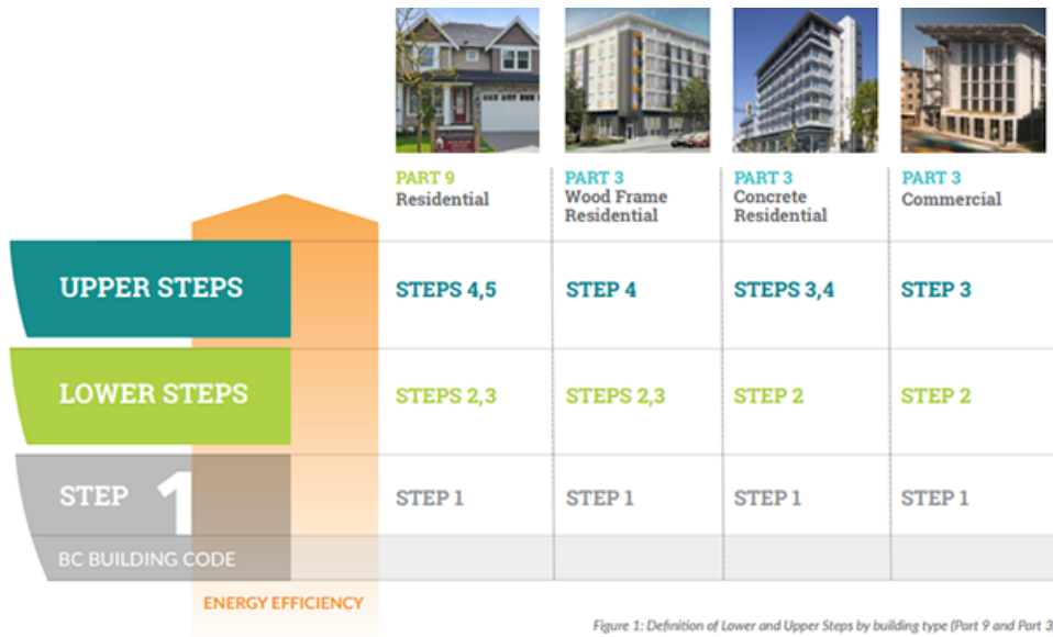
Figure 1: Definition of Lower and Upper Steps by building type (Part 9 and Part 3)
